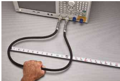
Flex Test (one full cycle)
